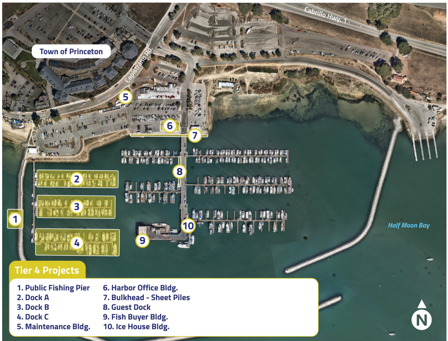
Figure 6. Pillar Point Harbor Tier 4 Projects, 2021
