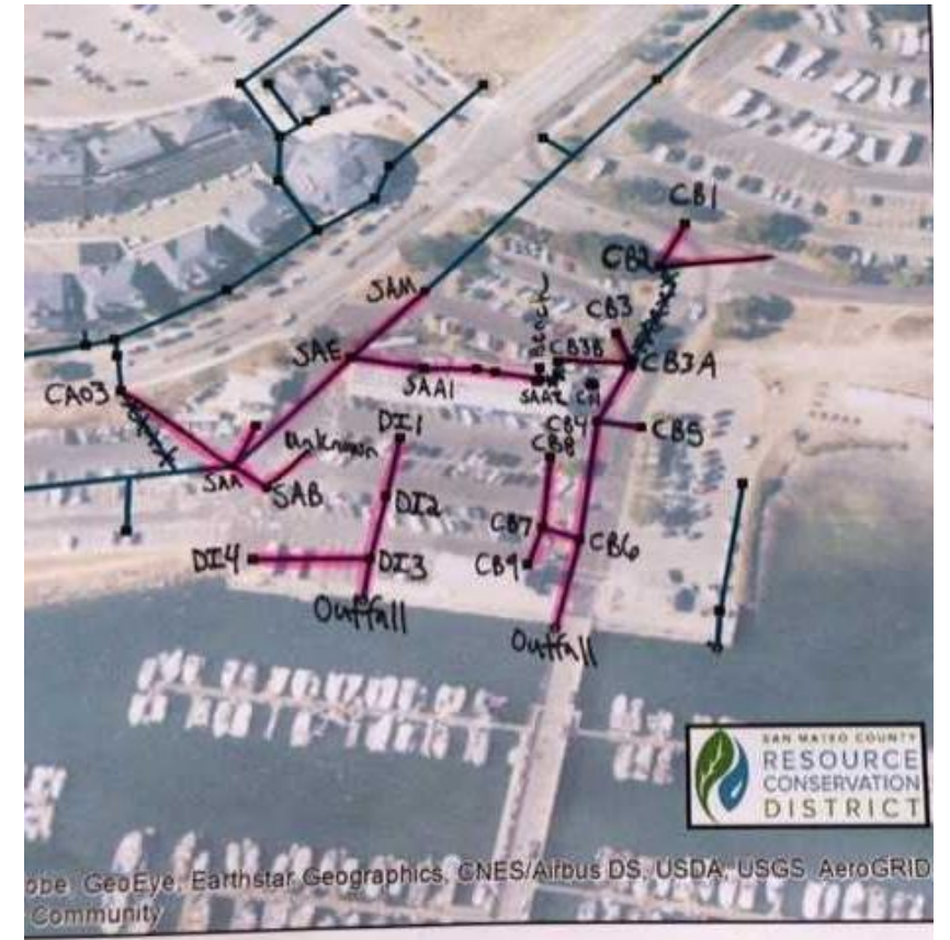
South Stormwater Lines
