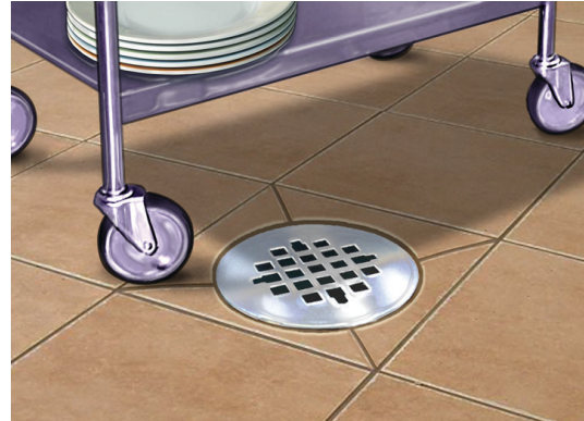
Sanitary Sewer Drain: An indoor drain that flows to the sewage treatment plant.
