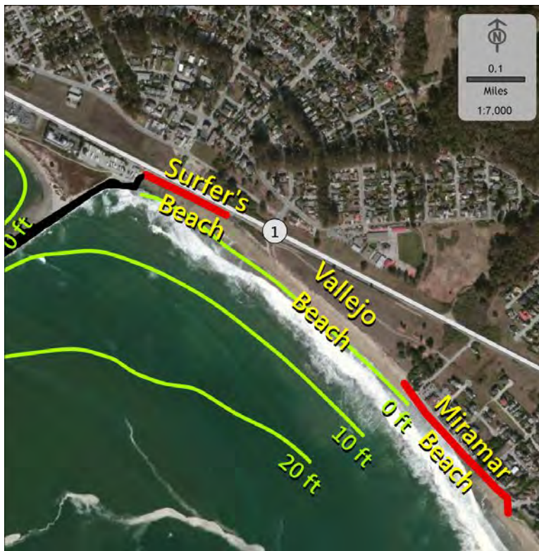
Figure ES- 2: Local beaches, root of the East Breakwater (black line), and revetments (red lines) Contour depths are relative to MLLW.
