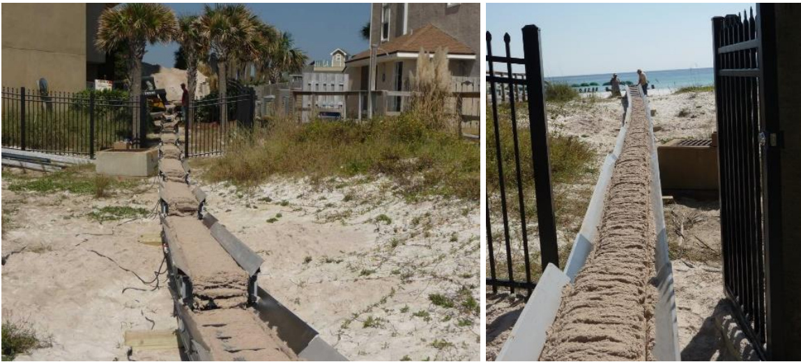
Figure 21 Portable conveyor system transporting sand
