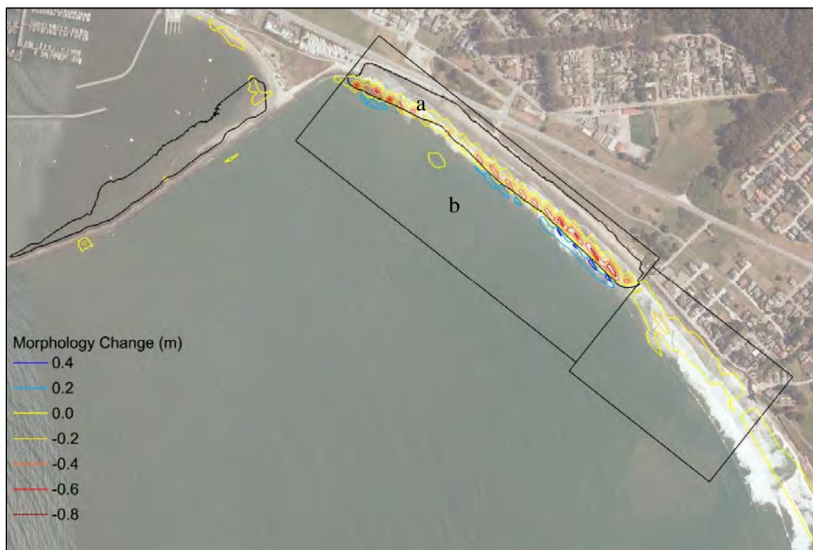
Figure 8. Modeled Erosion and Accretion in the Vicinity of Beach Fill Placement (140,000 to 150,000 CY) and Borrow Areas from June 2009 to November 2009 (6 months). (Source: Lin et al., 2015)
