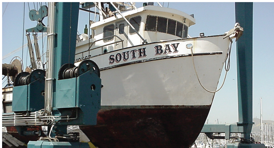
Photo: A travel lift moves the South Bay out of the water for maintenance repairs.
